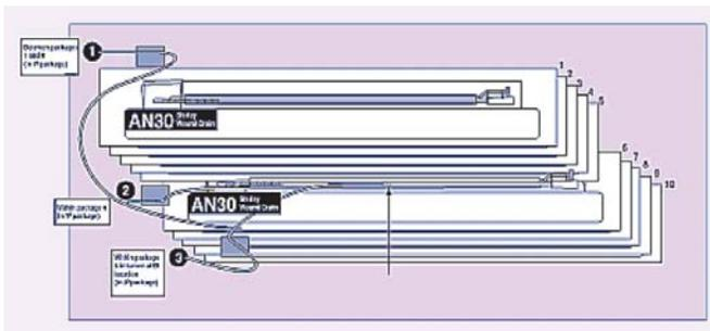
Figure 2. Temperature and humidity probes were placed in three product multipacks. The arrow indicates the worst-case biological indicator site.
